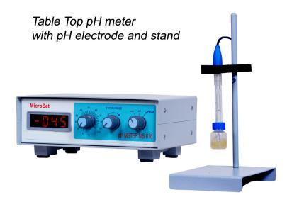
It is a high-precision pH meter for continuous 0-14 pH reading & milli volts. The pH meter is easy to operate as it has the least number of controls. CHECK facility saves time from every day buffer standardization and hence is most suitable for quick analysis. It is a very sleek attractive finished instrument.
