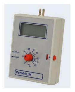
MS pH 816 is a compact Handy highly precision pH meter for continuous 0-14 pH reading & is easy to operate as it is having least number of controls. Auto Bat. Low Indication is displayed as BAT when battery voltage falls to 7.6 volts dc.
